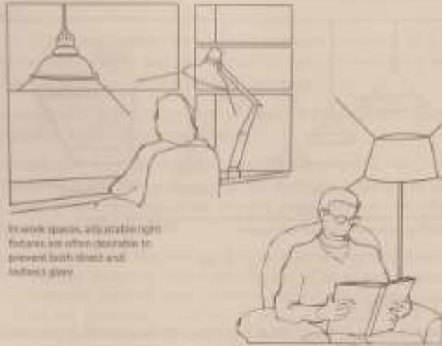
In work spaces, adjustable light fixtures are often desirable to prevent both direct and indirect glare.
